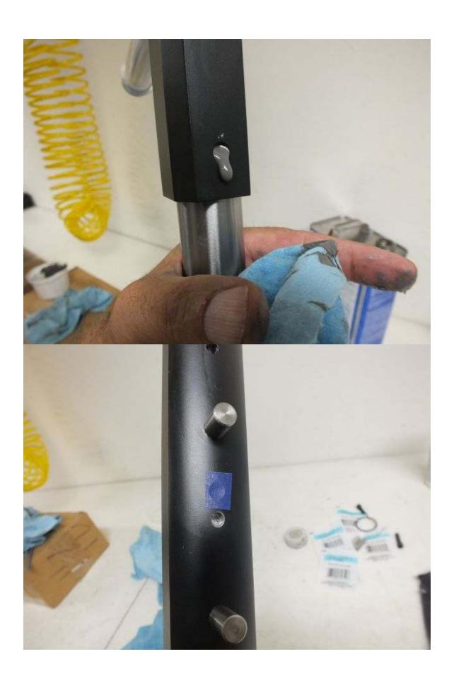
Re install assembly into chassis and tighten screws, using a quality level, level the forend (do not go off the top of the block) then level the action assembly off the scope rail, re check level frequently as the epoxy sets, the epoxy level in the sprue holes may drop as remaining air escapes, just drizzle a bit more epoxy into them as needed, insert a few cardboard shims snugly between the barrel and forend and allow the epoxy a minimum of 24 hours to cure.
