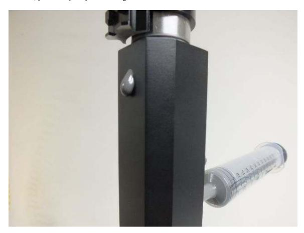
When complete block injection hole with a small piece of tape
