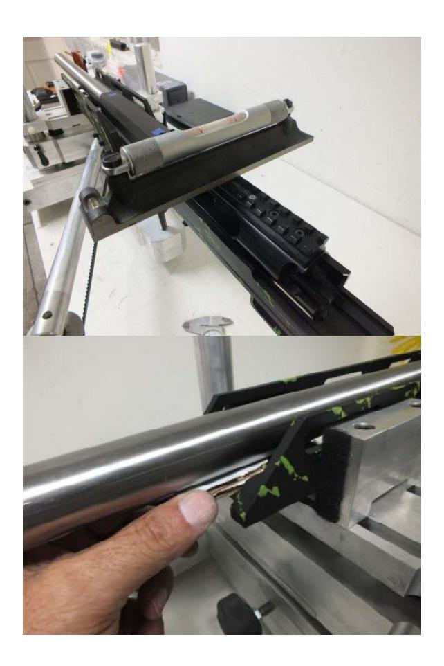
After epoxy has cured 24 hours remove the action assembly, install trigger and bolt and re assemble, note the location of the bolt handle notch and using a Dremel type tool carefully create clearance for the bolt handle, care must be taken to ensure the bolt handle does **not** contact the chassis in any way.
