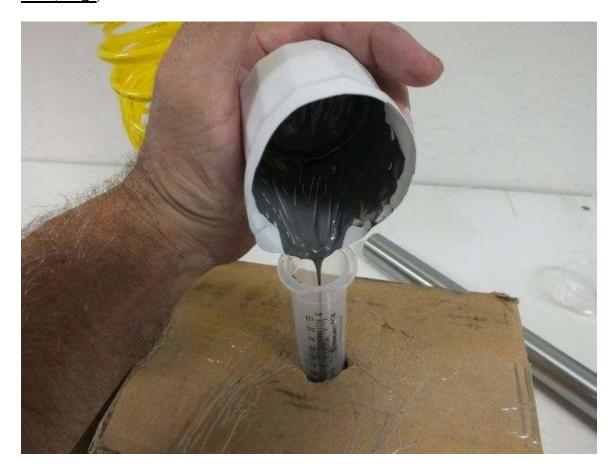
Install piston and invert syringe to purge all air form it before injection
