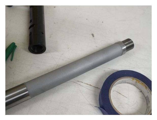
Install barrel to action and tighten securely
